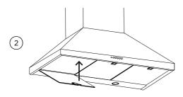
Place the filter into the support at the rear of the range hood. Push the filter back into place.
