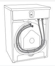
The water intake hose has to be fastened firmly enough for the hose to have a good seal. After connecting the hose, the seal must be checked for any leaks.
