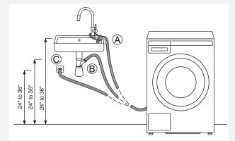
Drain hose can also be connected directly to the washbasin drain via a siphon. In this case, the hose, too, should be 24" to 36" mm above the floor. Internal hose diameter should be at least 18 mm. See figure.
