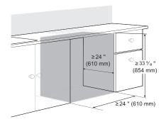
2 To allow for proper clearance of plumbing and electrical, use the template included with the literature to determine the clearance on the side of the cabinet where the cabinet meets the back wall. Using a 2 1/2" diameter hole saw, drill a hole in the target area as shown on the template.
