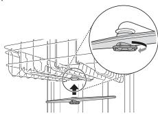
After assembly, make sure that the spray arms rotate freely.
