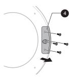
Swap the position of the hinge assembly 3 and the door latch assembly 4 and reassemble. Refer to steps 2 and 3 for the location and number of screws when reassembling.
