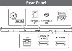
DC IN······AC adapter input OPTICAL IN·····Connect to an optical device. PORTABLE IN·····Connect portable device. USB (Service only) ·····S/W download connector. LAN·····Connect to router. HDMI OUT (TV ARC)····Connect to a TV. HDMI IN······Connect to device with HDMI OUT.
