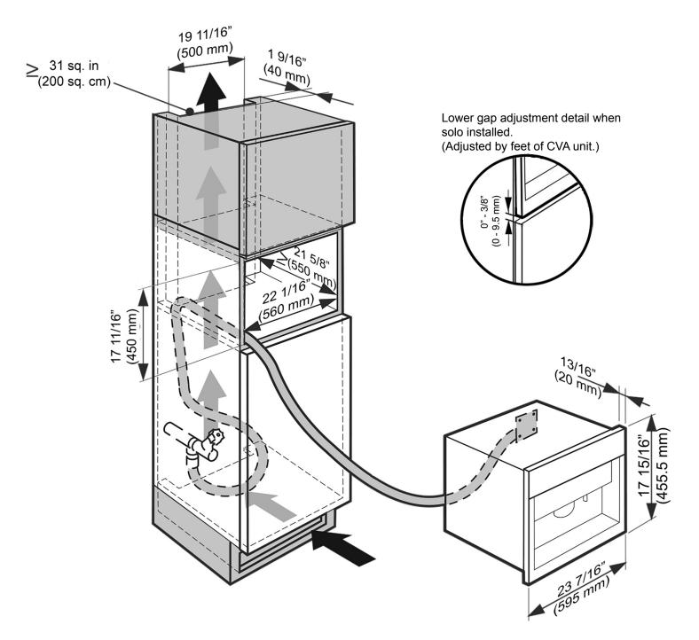
**PLEASE NOTE:** Condensation water can damage the coffee system or surrounding cabinets. The specified ventilation cross-sections absolutely must be observed.
