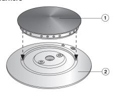
■ Place the burner cap ① on the burner base so that the lobes on the burner cap engage in the holes in the burner base.
