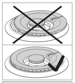
Burners cannot function correctly if they are incorrectly assembled. This can lead to damage to the appliance and injury.
