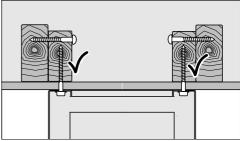
The hood must be attached to rigid structural framing that is supported in its entirety by the ceiling joists, or to the ceiling joists directly. Do not attach the plate directly to the ceiling with anchors, toggle bolts, etc.
