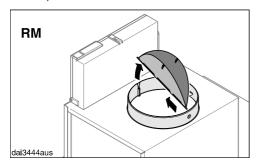
■ With vented mode (AE) insert the non-return flap in the exhaust socket if your ducting system is not equipped with one.
