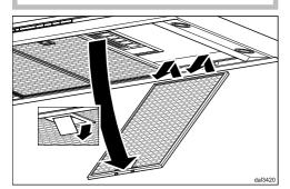
■ To remove a grease filter, release the locking clip. Then, open the filter to a 45° angle, unhook it, and remove it from the hood
