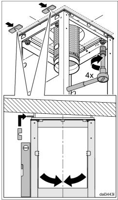
Align the installation frame and secure it with the screws. The spacers, which were removed from the spacer frame at the start, can be used to align the hood vertically.
