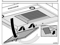
■ To remove a grease filter, release the locking clip. Then, open the filter to a 45° angle, unhook it, and remove it from the hood.
