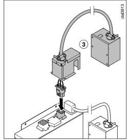
■ When using an external blower, the connection box ③ of the external blower is plugged into the appropriate socket on the connection box.
