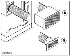
Connect the DUU 2900 recirculation box (A) to the exhaust socket.
