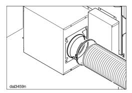
Secure the exhaust ducting to the exhaust socket, e.g., with a hose clip (available as an optional accessory) on flexible ducting.
