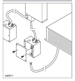
Install a connection cord from the downdraft to the external blower. Refer to the Operating and Installation Instructions for the DAG 1000 external blower.
