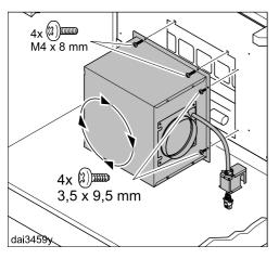
Rotate the motor so that the exhaust connection points in the required direction and secure it to the downdraft.
