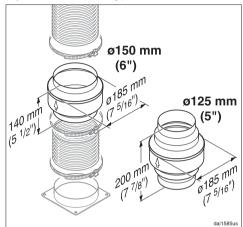
In addition to appropriate insulation of the exhaust ducting, we recommend installing a condensate trap to collect and evaporate any condensation which may develop. This is available for ducts  $\varnothing$  5" ( 125 mm) or  $\varnothing$  6" ( 150 mm).
