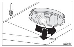
■ Turn the light counterclockwise and pull it out.
