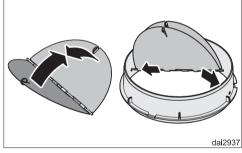
■ If required, insert the non-return flap. Ensure that the flap opens easily and closes by itself.
