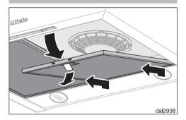
Open the grease filter locking clips and pull the filter down to remove.
