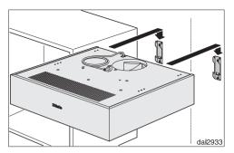
Attach the hood to the wall anchors.
