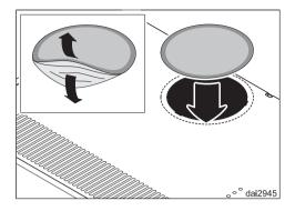
■ For operation in recirculation mode, cover the opening at the back with the sticker.
