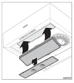
■ Reinsert the cover and the grease filter.
