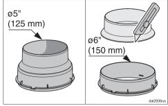
■ For an Ø 6" (150 mm) exhaust duct, use a pointed knife to cut off the exhaust collar where it tapers. For an Ø 5" (125 mm) exhaust duct, use the collar as is.
