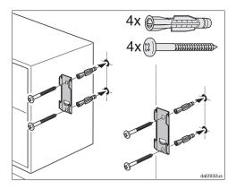
■ Fasten the wall anchors to the wall using the dowels and screws provided.
