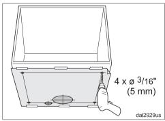
■ Drill four mounting holes Ø <sup>3</sup>/<sub>16</sub>" (5 mm) through the bottom of the cabinet.
