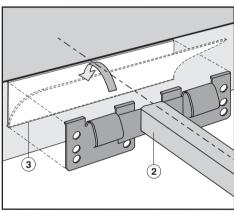
■ Position and attach the spring clips
