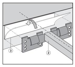
Position and attach the spring clips
