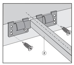
Place the supplied spring clips ① and the support bars ② at the marked positions as shown above, by laying them on the upper edge of the cut-out and then securing them with the <sup>1</sup>/<sub>8</sub>" x 1" (3.5 x 25 mm) screws (supplied).
