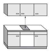
The minimum safety distance given by the hood manufacturer must be maintained between the combiset and the hood above it. See the installation instructions of the hood for these safety measurements.
