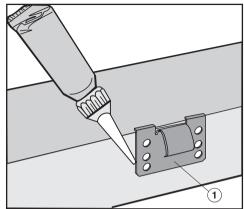
Coat the side and lower edges of the spring clips between (1) and (2) with silicone.
