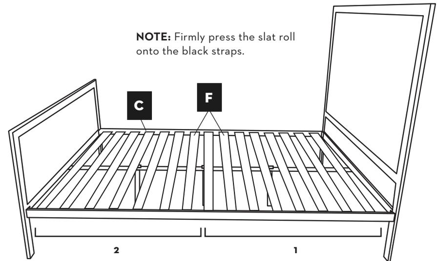
**NOTE:** Firmly press the slat roll onto the black straps.
