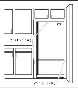
To ensure proper ventilation for your refrigerator, allow for a  $\frac{1}{2}$ " (1.25 cm) space on each side and at the top. Allow for 1" (2.54 cm) of space behind the refrigerator. If your refrigerator has an ice maker, allow extra space at the back for the water line connections.
