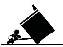
To reduce the risk of the appliance tipping, it must be secured and connected using the anti-tip device according to the installation instructions. Re-engage the anti-tip device if the range is moved.
