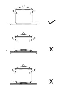
The pans must have certain minimum diameter to ensure optimal operation. Pans larger than the cooking zones can also be used: make sure that the bottom of the pan does not touch other cooking zones and that it is always centered over the inductor.
