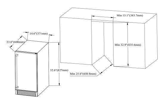
When installing the ice maker under a counter, follow the recommended spacing dimensions shown. Allow at least 2" (50.8 mm) of clearance at rear, and  $\frac{1}{4}$ " (6.35mm)at sides for proper air circulation.
