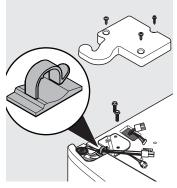
3. Release the wires from the routing clip.
