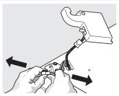
Disconnect the multi-wire cable connector located above the top hinge. Press the cable and lock and separate the 2 cables.
