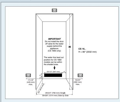
The appliance can be used freestanding or semi built-in. If semi built-in, consider the cabinet opening dimensions.
