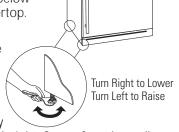
1/8" less than the opening height. Screw front legs all the way in to shorten the height at the front. This will allow you to slightly tip the unit into the opening. Once in the correct position, the front legs can be adjusted to level the product.
