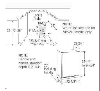
For a standard installation: The product must be installed so that the stainless steel front will project 1-5/8" forward of adjacent cabinets. This position will allow a full door swing and prevent interference with adjacent cabinetry. The opening between cabinets must be 23-3/4" minimum.
