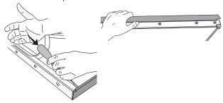
Remove 4 screws to remove the top door trim (do NOT discard).
