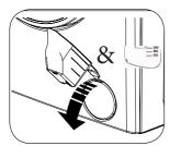
• You may use the washing powder spade supplied with your machine or liquid detergent level plate to open the pump cover.
