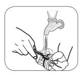
• Clean the foreign materials inside the Iter with the help of a brush.
