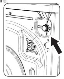
Remove the filter of the water inlet valve on your machine with a pair of pliers. Clean thoroughly using water and a brush.
