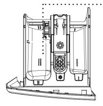
Main wash detergent compartment: In this compartment, only materials like detergent (liquid or powder) or anti-lime. You can find the liquid detergent apparatus for your liquid detergent inside your machine during the first set up.(\*)
