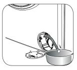
• Pull the black rubber hose and detach it from its clamp, place a container under it and remove its plug.
