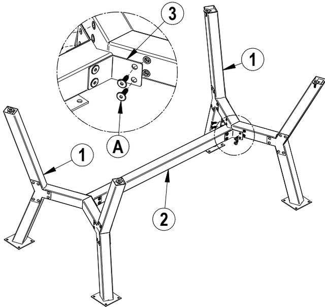
3) Screw on lightly plates **3** on the legs **1** with bolts **A**.
