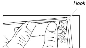
6. Reattach the second top vent cover with the screw removed in step 1.
