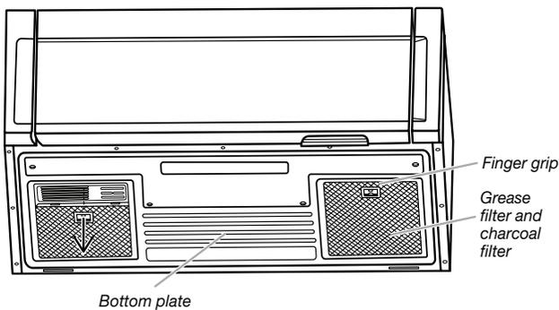
2. Separate the grease filter from the charcoal filter.
