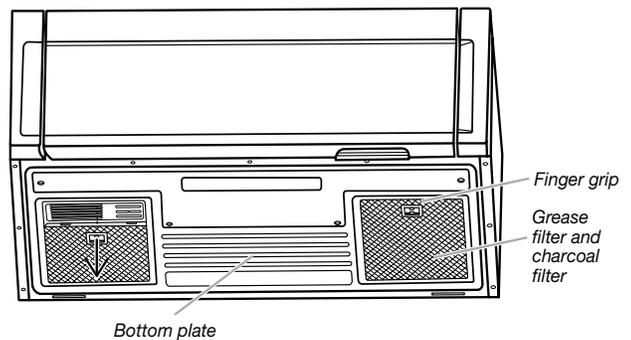
2. Separate the charcoal filter from the grease filter.
