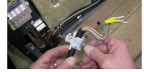
4. Insert the strain relief device into the hole and push it to the left. Tight up the power cord and strain relief device with the screw.
