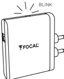
The LED is blinking : the receiver is powered, no source is associated, you can associate a new device.
