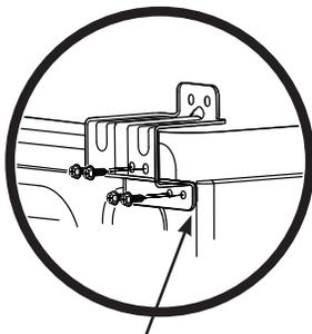
Install brackets flush at washers edges
