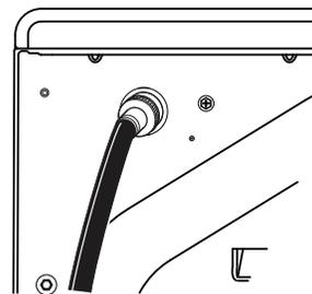
7. Using pliers, tighten all the couplings with an additional two-thirds turn.
