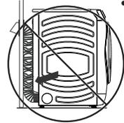
• **DO NOT** crush duct against the wall.
