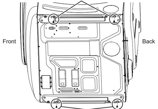
Attach spacer using 2 screws
