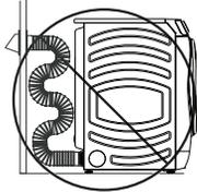
• **DO NOT** use excessive exhaust length. Cut duct as short as possible.
