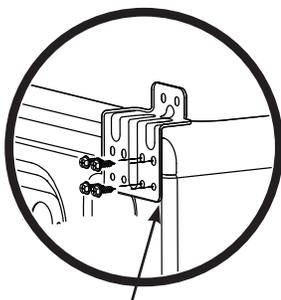
Install brackets flush at washers edges
