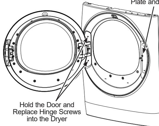
Hold the Door and Replace Hinge Screws into the Dryer
