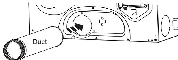
**NOTE:** We strongly recommend using rigid metal exhaust duct. However, if flexible ducting is used it must be UL-Listed metal, not plastic.
