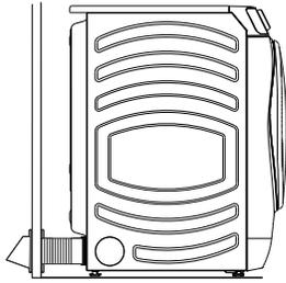
• **DO** cut duct as short as possible and install straight into wall.
