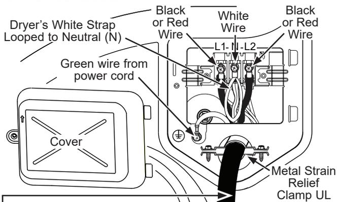
4 #10 AWG minimum copper conductors or 120/240V 30A power supply cord kit marked for use with dryers and provided with closed loop or spade terminals with upturned ends (not supplied).
