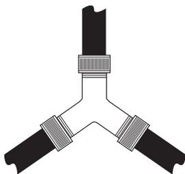
4. Insert the filter screen in the coupling of the **washer's** inlet hose. If a rubber flat washer is already in place remove it before installing the filter screen. Attach this coupling to one male end of the “Y” connector. Tighten by hand until firmly seated.
