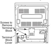
For power cord and 1" conduit only, remove B the knockout ring (13/8") located on bracket directly below the terminal block. To remove the knockout, use a pair of pliers to bend the knockout ring away from the bracket and twist until ring is removed.
