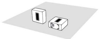
Make sure at least one side of the rectangular opening (acoustic slot) is unobstructed.
