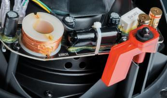
**PRECISION-BUILT, ADVANCED TOPOLOGY VOJTKO™ CROSSOVERS.** Carefully hand-built using only the finest polyester capacitors and air-core coils, Installer Series crossovers employ MartinLogan's proprietary Vojtko topology for vanishingly low distortion and seamless driver integration. This precisiontuned network preserves even the most microscopic sonic nuances while handling the full dynamics of any source.
