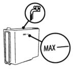
② RINSE AND FILL WATER TANK UP TO MAX LEVEL: Fill the tank up to the MAX level with fresh water.
