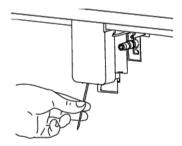
② Check that the holes in the coffee spouts are not blocked. If necessary, remove coffee deposits with a toothpick.
