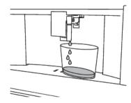
② PLACE 2L CONTAINER UNDER SPOUTS PRESS ✓ TO START DESCALING: Place an empty suitably sized container under the steam wand and coffee spouts.
