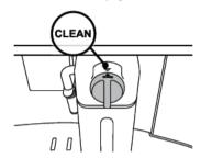
③ Turn the froth adjustment dial to CLEAN, CLEANING MILK CONTAINER UNDERWAY appears on display.
