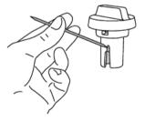
(§) Wash all the components of the frother thoroughly with hot water and dishwashing liquid. All components and the container are dishwasher safe. Make sure there are no milk residues on the hollow and groove under the dial. If necessary, scrape the groove with a toothpick.
