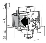
Safter cleaning, replace the infuser by sliding it onto the internal support and pin at the bottom, then push the PUSH symbol fully in until it clicks into place.
