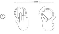
Push the dial in and turn counterclockwise to HI. Hold the dial at HI before turning to a flame setting.
