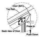
STEP 2: Use your forefingers to press in the buttons at the side of the Latches and then Press down the buttond of door. If the latches are at lower position already, please take out the door.
