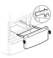
Lower the door into its final position and insert the screws in the rails on both sides.
