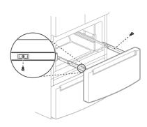
Grip both sides of the drawer and pull it up to remove it from the rails.
