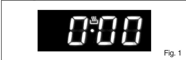
“Auto” and “0:00” will start flashing when the unit is switched on for the first time. To set the clock, press the central button for about 3 seconds. When
