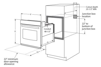
Electric wall ovens are not approved for installation with a plug and receptacle. They must be hard wired in accordance with installation instructions.
