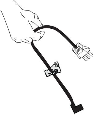
Remove the Power Cable with grounded lead and Connector from the Rangehood.
