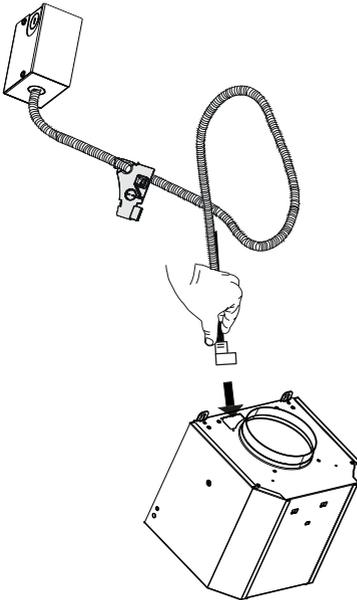
For Rangehoods with an easy cube, insert the motor connector in the wiring hole where the previous wire was taken out.
