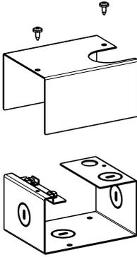
Open the Cover of Wiring Box by unscrewing the two screws.
