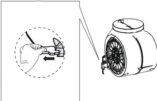
For Rangehoods without an easy cube, disconnect the power cable from the motor directly.
