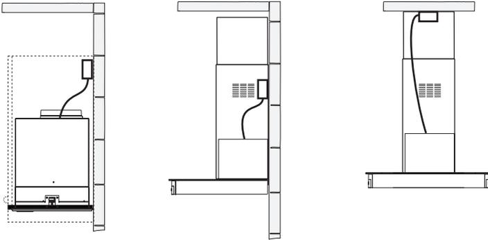
The Wiring Box can be installed on the wall, in the cabinet, or in the ceiling depending on the specific rangehood model and power connection in the house.
