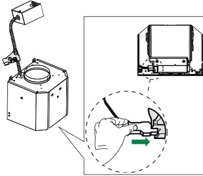
Reconnect the Motor Connector to the blower (both types shown).
