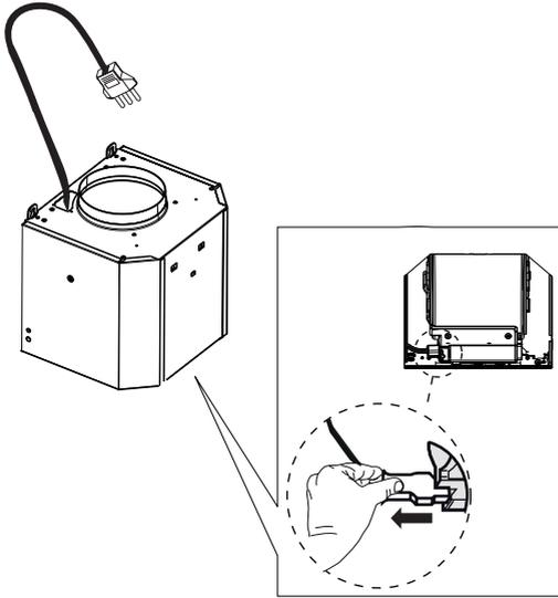
For Rangehoods with an easy cube, disconnect the power cable from the motor inside the motor box.
