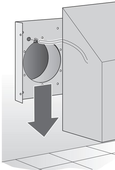
5. Screw the fan onto the mounting plate.
