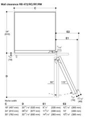
The drawing is based on a cabinet panel width of  $^{3}/^{4}$  (19 mm) and a Gaggenau cabinet handle height of  $1^{5}/_{10}$  (49 mm).
