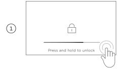
Press and hold anywhere on the screen until the bar fills and the oven unlocks.
