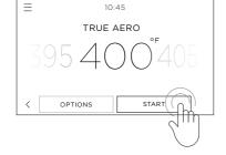
After 5 minutes, change the function to **TRUE AERO** and heat for a further 20 minutes. When you have finished, turn the oven off.
