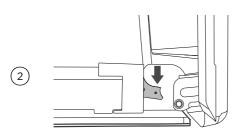
Ensure the door is firmly in place on the hinges. Open the door fully again and push each locking lever down to lock the door onto the hinge.
