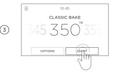
To adjust the preset temperature, swipe left or right or use the dial. Touch **START** to heat the oven and begin cooking.
