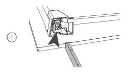
Holding the door on both sides, line up the holes in the base of the door with the hinges and slide the door on.
