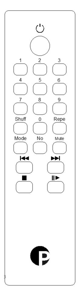
Button on top turns the unit on or back to standby. (The lever switch must be in the up position)
