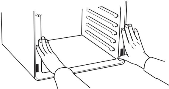
4. Securely fasten oven to cabinet using the two 4 x 25 mm self-tapping screws provided. Insert the screws through holes in mounting rails. Do not overtighten screws.
