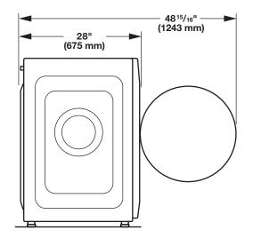
All dimensions show recommended spacing allowed, except for closet door ventilation openings which are the minimum required.
