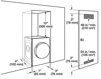
**NOTE:** The 12" minimum space above the washer/dryer is required for use of the Load &  $Go^{M}$  bulk dispenser.
