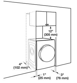
**NOTE:** The 12" minimum space above the washer/dryer is required for use of the Load &  $Go^{M}$  bulk dispenser.
