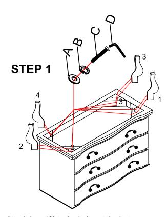
Attach legs (2) to the holes at the bottom corners of case body (1), tighten all with flat washers (A), lock washers (B) and bolts (C) by using allen wrench (D).
