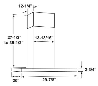
30"models require a 30"-wide opening \*The supplied duct cover fits 7'-7" to 9'-6" ceiling heights (10' ceiling height with optional high celling kit UX10DC8SLSS) (12' ceiling height with optional high celling kit UX12DC9SLSS) (14' ceiling height with optional high celling kit UX14DC9SLSS)
