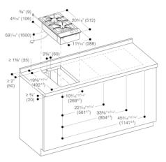
Minimum distance from the appliance cut-out to the side wall  $11^{13}\!/\!{}_{10}{}^*$  (300 mm). Measurements in inches (mm)
