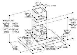
With the exhaust air duct cover AD 442 016 suitable for ceiling heights of 7.6 ft (2.35 m) to 8.6 ft (2.60 m).
