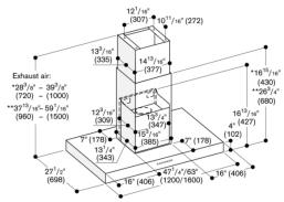
With the exhaust air duct cover AD 442 016 suitable for ceiling heights of 7.6 ft (2.35 m) to 8.6 ft (2.60 m).
