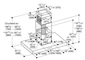
With the air recirculation duct cover AD 442 116 suitable for ceiling heights of 7.6 ft (2.35 m) to 8.6 ft (2.60 m).
