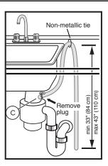
Note: Plumbing installations will vary - refer to local codes. Drain hose included is 79" (201 cm) and can be extended to a maximum of 155 3/4" (396 cm).
