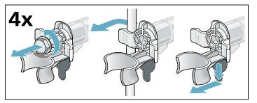
**3.** Place covers over the transport bolt holes. Four plastic covers are provided in the small parts bag included with your washer. Separate these covers and install one in each hole where the transport bolts were removed.
