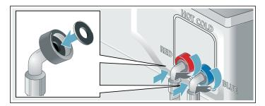
Attach this end of the hose to the back of the washing machine. Hand tighten only.
