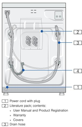
4 Elbow to form the hose to fit the drain pipe
