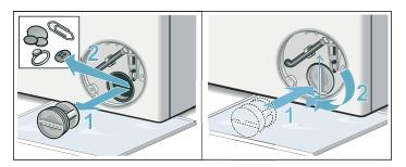
6. Turn the pump cover counterclockwise to remove it. A small amount of residual water may flow out when the cover is removed.
