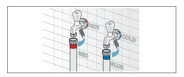
Attach this end to water tap. Hand tighten only.
